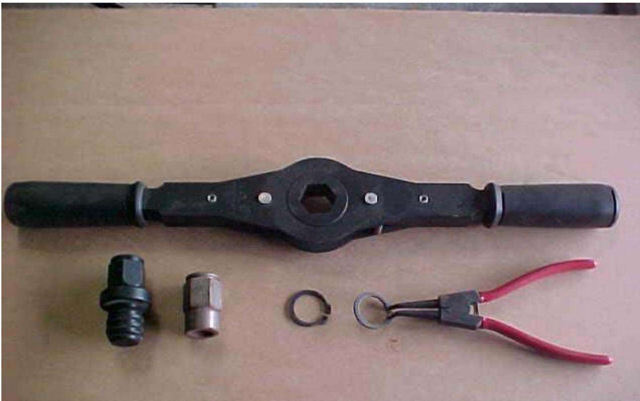
AMS ratchet T-handle modification to suit Dormer coarse thread. New centre is on left, then old centre, then existing circlips (only 1 circlip needed to secure new centre because has flange above male thread). Item code ADAPT(AMS).
