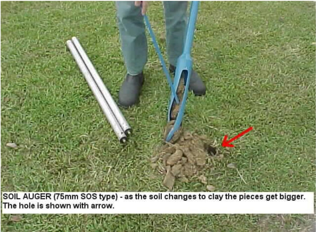
**SOIL AUGER (75mm SOS type) - as the soil changes to clay the pieces get bigger. The hole is shown with arrow.**
