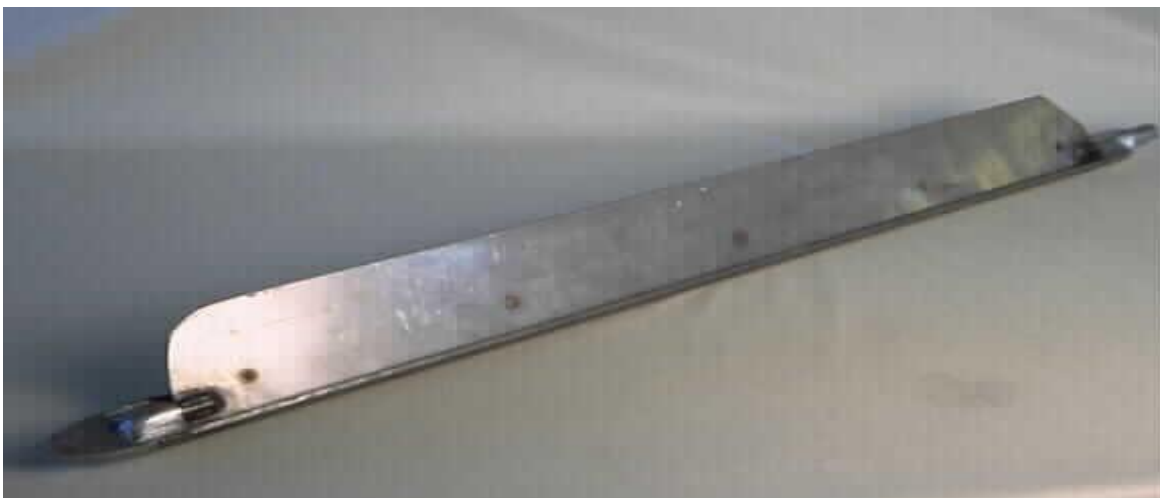
Russian D-sampler - for very soft wet samples. Made of SS.
