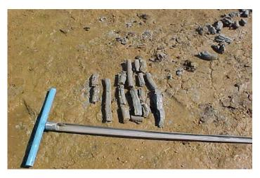
The sample can be removed in pieces when the material is plastic enough by inserting a spoon or blade and sliding sections of sample toward the bigger end. An old spoon is very useful when removing sample and a narrow, long bristled, stiff brush is very useful for cleaning.
