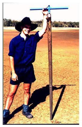
This is a 73mm x 1.8m long Gouge Auger we made for a hydraulic push rig which was now being used by hand in mangrove mudflats in North Queensland where the rig could not access.
