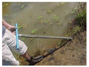
The sample profile can be viewed and logged against the 100mm increments cut into the edge of the sampler. For more accurate assessment the surface should be cut away to remove any contamination from the side of the hole as it was pulled out (the taper reduces this problem). Be very careful of the sharpened edges when handling the sampler, removing sample or cleaning it.
