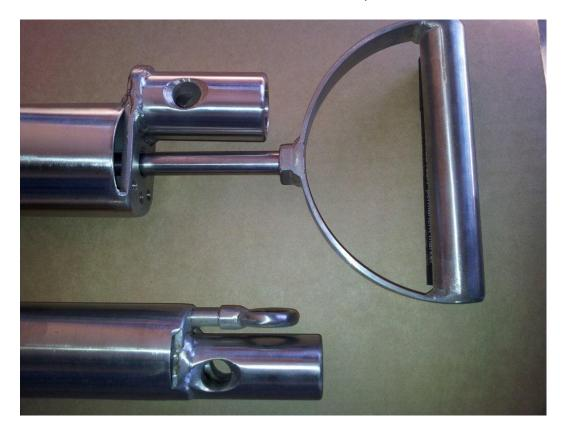
The rope loop on bottom one in pic is standard and the D-handle shown on top one in the pic is an optional extra (both are threaded on).
